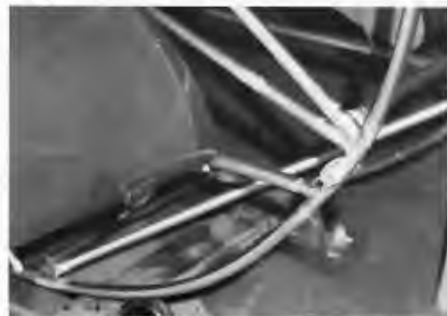
Figure 2. View of hoop splice and forward wing attach point. Cradle frame is made of 2 by 4's bolted together.
