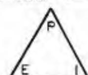
Cover the unknown with your finger. The visible remainder is the equation to calculate the unknown, e.g. E = IxR; E = P/I.
