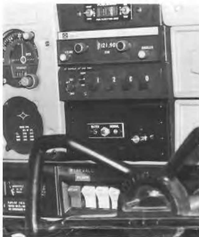
Here we can see the "water in fuel" indicator in the panel of the Piper Cherokee being used as an auto fuel test aircraft by the EAA Aviation Foundation.
