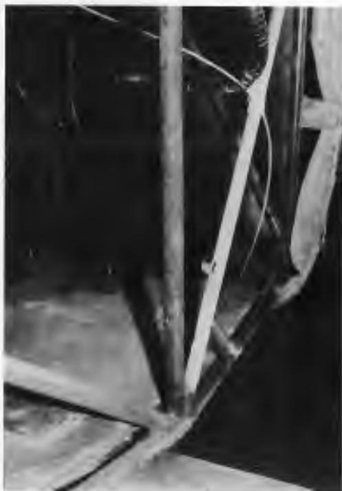
The pictures do not show how badly this particular tube is rusted. This tube is the one at the front door post and a consensus here is that it has lost nearly 50% of its wall thickness due to the heavy scaly rust. A sharp punch easily punctures the wall of the tube. If this tube breaks, the lower strut assembly acts like a fulcrum, and there goes your wing.
