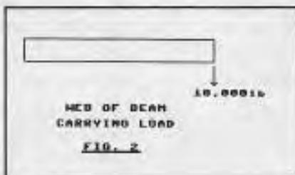
web must be in equilibrium. Since we are supporting 10,000 pounds, and the web carries the load, the load is pulling down on the web with a force of 10,000 pounds. This can't be in equilibrium, since there is no equal and opposite force. But the only place we can have a force pulling up is at the wall (fig. 3).
