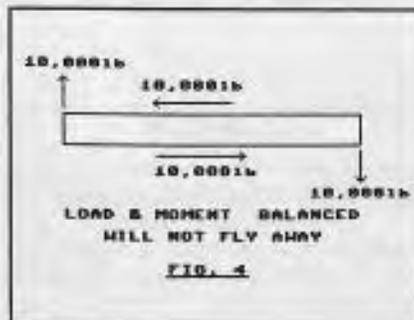
However, to choose the attachment of the caps to the web we want to distribute the forces evenly along the span, so we generally think of the forces in pounds per inch. Since the beam is 100 inches long, the force per inch would be 100,000/100, or 1000 pounds per inch. We call this the **shear flow** (9). We could think of this as a load of 1000 pounds applied every inch, or a force of 500 pounds every half inch, depending on how far apart the fasteners are.
