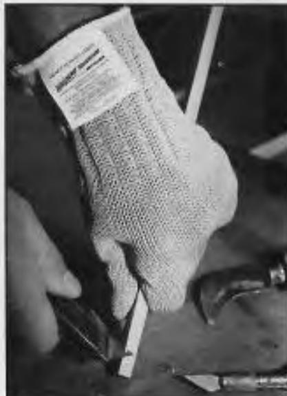
This is a whittler's glove and it has steel strands imbedded in the glove to protect the craftsman from sharp objects. It will fit either the left or right hand and is available in hardware stores and fishing supply stores locally.
