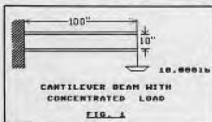
100 inches long, and is supporting a load of 10,000 pounds at the end. Of course an actual wing will have a distributed load all along the span. We will consider that later.
