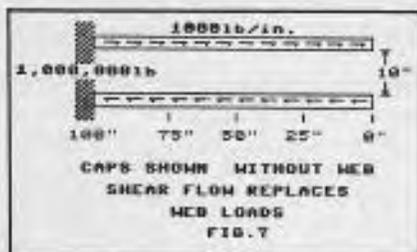
and show them in equilibrium (fig. 7), the 9 is applied to the caps by the web, the 9 along the top cap is shown acting to the right, because it was acting to the left in the web. (opposite reaction) Since each load is acting in the same direction on the cap, the loads are adding to each other so that
