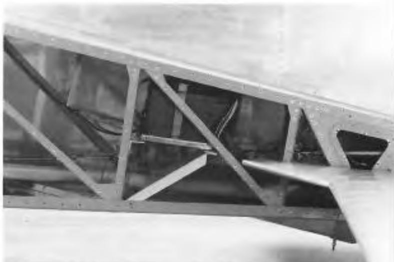
The fuselage has been stretched 18 inches to accommodate the large engine and it was necessary to place the battery at the leading edge of the horizontal stabilizer in the aft fuselage.
