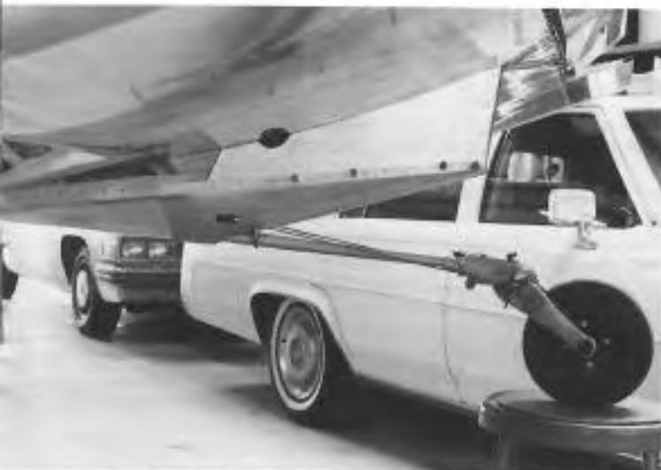
The tailwheel spring is round, like a 185 Cessna, and is faired into the fuselage.
