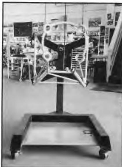
This stand was built to hold the mount and engine until the fuselage is finished. This may also be the cleanest shop I have seen pictures of in quite a while.
