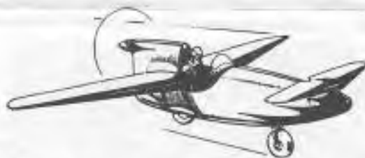
BELTRAME "COLIBRI" 18-h.p. Beltrame engine. This interesting tail-first light plane is of Italian origin.
