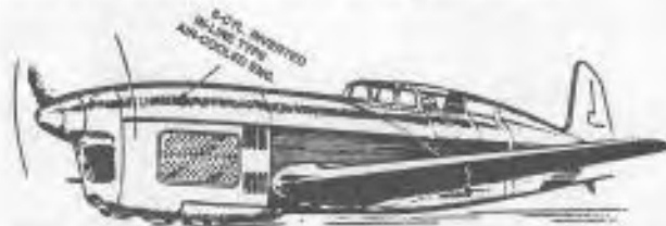
CAUDRON C-46 RACER 340-h.p. Renault air-cooled in-line engine set a new world's record for landplanes at 314 m.p.h., and although it had about half the power of the other competing aircraft, it won the 1936 Thompson Trophy races at 264 m.p.h.
