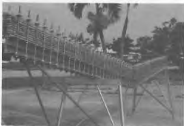
Corby Starlet spar jig, 1 piece wing spar still in the jig. Being built by Newsletter Editor, Vic Boyce for "Ole" Oleson of Reno Nevada.
