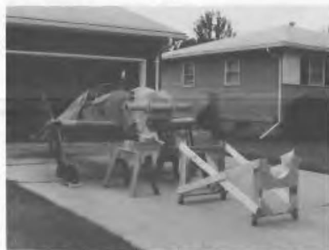
We see the airplane sitting on its landing gear and inverted cradle positioned in front of the airplane, ready to be turned over.
