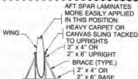
to a base with a heavy carpet sling between the two upright boards. The weight of the wing pulls the boards together and stabilizes the whole jig. It would probably be a good idea to make some angle braces for the uprights, also.
