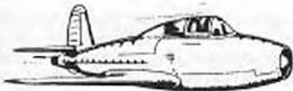
GLOSTER E.28/39 First Allied plane to be jet-powered. This was not a service fighter but a flying test bed for the new Whittle jet engine.
