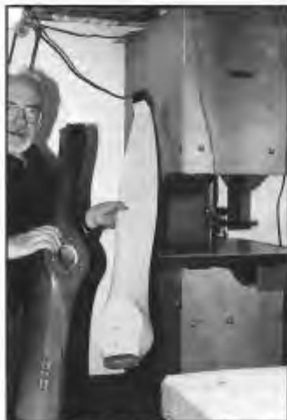
This shows Al Clark's prop duplicating machine-homemade and in the background the Lemie bandsaw which uses Volkswagen wheels and spindles giving it a 24 inch throat. The prop carving machine he calls a kite machine and we are asking him for more details. Also shown is the layout and fuselage welding table for his tailwind.
