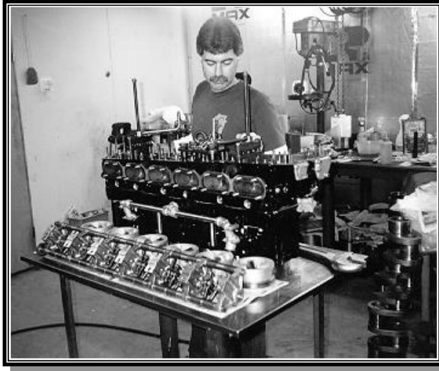
Rick inspecting a cylinder/cam assembly before mating it with the case
