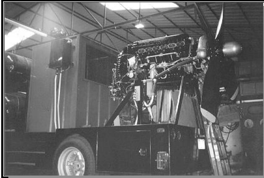
A Merlin almost ready to run, mounted on the 1964 International test stand
