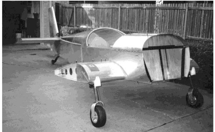
fiberglass dorsal fairing for the tail, and the formed Plexiglas canopy. Vern will probably build the canopy frame himself. It won't be long before the fuselage is ready to be joined with the completed wings at AeroCountry.
