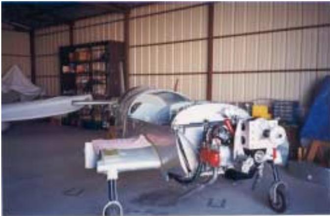
The engine is an 1800 cc Subaru EA81 flat four. The engine was imported from Japan. Prior to its installation Vern did a careful inspection of the engine. He reports that the drained oil was clean, the oil galleys had a nice light brown color, and the hone marks were still visible in the cylinders. Vern has installed a two barrel carburetor, a small alternator, and a small flywheel. The engine was rated at 79 HP stock. Vern is looking to get five additional HP out of it.
