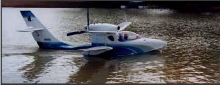
This is a real success story of how Tom took the old Sea Hawk design and turned it (major redesign) into the Glass Goose, which is a real performing aircraft as demonstrated both on and off the water. The Glass Goose now in production is being produced from new molds, using the latest state-of-the-art materials, and with the benefits of up-to-date computer modeling to verify important parts of the design.
