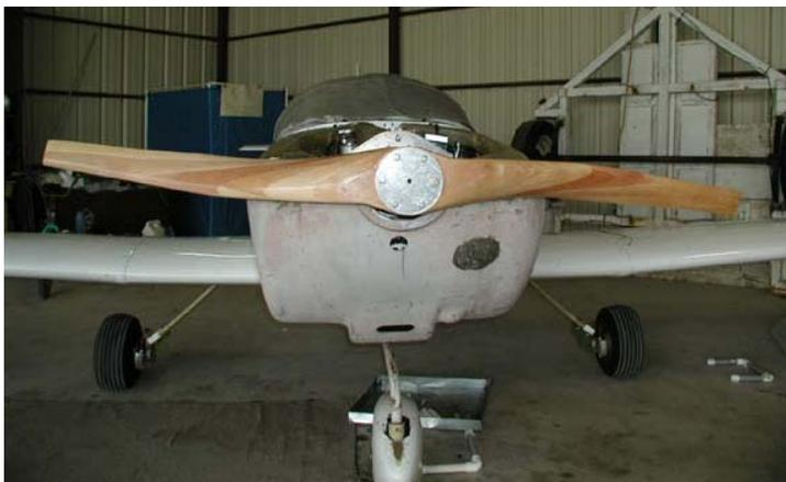
Now to the performance. Keep in mind that the current KR2 does not have any fairings for the wide main wheels. On an 80 deg F day, at 2000 ft MSL, climb rate was 1800 fpm at 110 mph. Max speed was 165 mph at that altitude, with the engine turning 5100 rpm and the propeller turning 2700 rpm. Cruise speed was 150 mph at 4800 rpm for the engine and 2500 rpm for the propeller.
