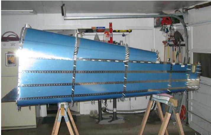
Unlike most RV kits, the tail kit consists of not only the tail feathers, but also includes the back half of the fuselage. Van's arranged it that way to even out the prices of the four sub kits. While studying the tail it is not hard to notice how much larger this airplane is than the other RVs. The horizontal stabilizer is as long as one of my RV-8's wings. I thought building one elevator trim tab was enough, but this one has two to
