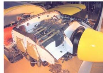
The reason for the markedly increased “oil consumption” was stuck scraper rings on two pistons. Amazingly, there was no spark plug fouling, presumably because of my electronic ignition. The engine’s “guts” checked out very well and went back together with “standard size bearings”
