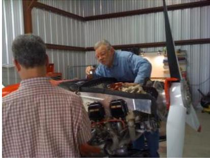
So, I was just as excited to see him pass that final hurdle before the airplane flies. He spent weeks before the inspection checking and rechecking for loose bolts and jam-nuts. We looked over clamps, safety wire, and things that might not pass inspection. We weighed the airplane.
