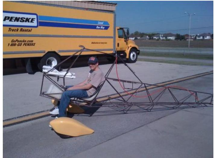
The Airbike has an empty weight of about 350 pounds and a gross weight of 560. It cruises at 65 mph and lands at 25mph. It uses 40 hp to lift it into the air, and the pilot straddles the fuselage and sits behind the engine.
