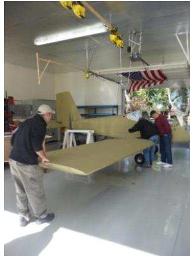
David lifted one end, Bruce lifted the other, and they slid it into the fuselage. It slid right in, and with 2 twists inside the fuselage, the two locking pins were in, and the job was done. It took me longer to type out
