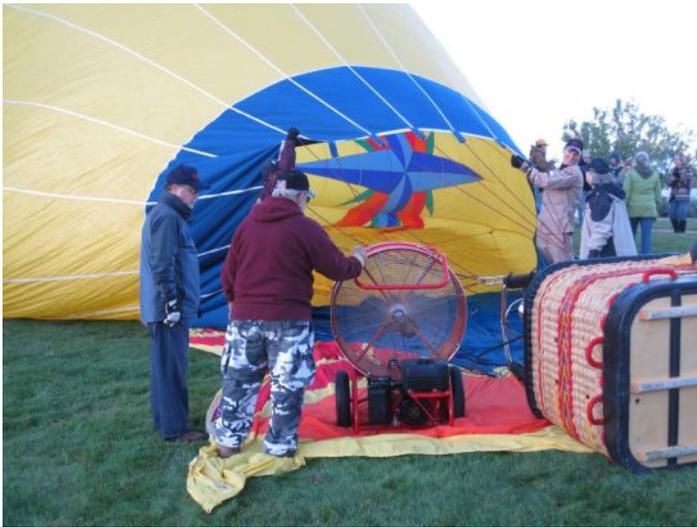
Once the fan has filled the balloon with air as much as possible, the burners of the basket are intermittently turned on, blasting flames into the hull.
