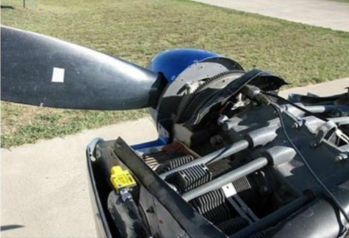
Not my plane, but the setup is the same. The optical tach sensor is yellow and mounted on the pilot side, and it picks up the white tape on the back of the prop. You can see the wire running to the vibration sensor mounted on the top center of the engine. Photo courtesy of [www.ExpAircraft.com](http://www.ExpAircraft.com)
