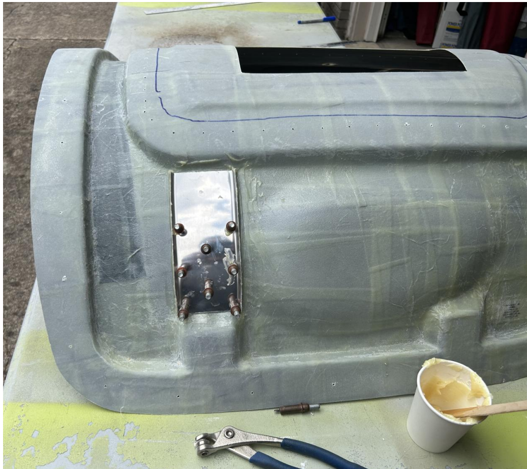
Attaching the hinge bracket support on the inner shell
