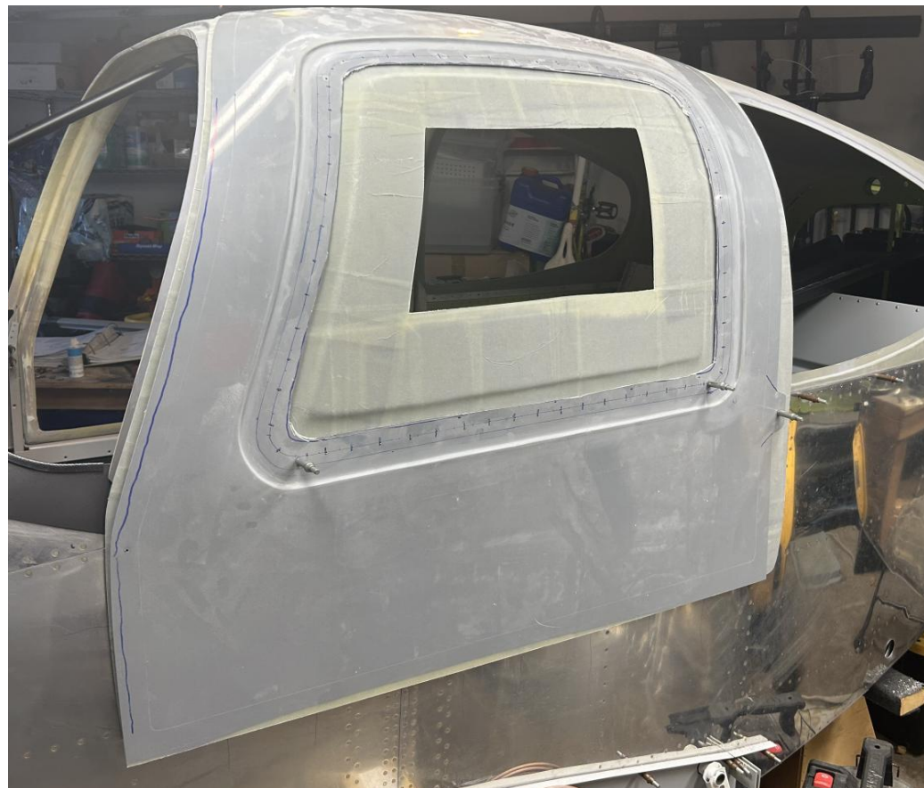
Attaching the inner and outer door panels with the fuselage cabin
