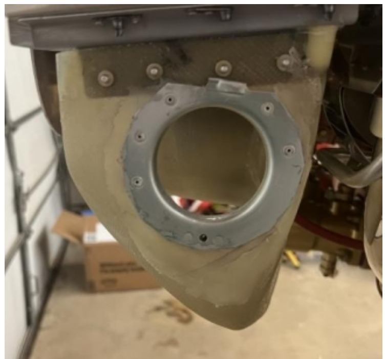
Alternate air intake installed
