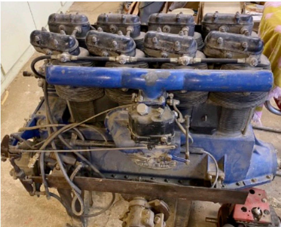
Menasco D-4 inline inverted 4-cylinder engine 125 HP
