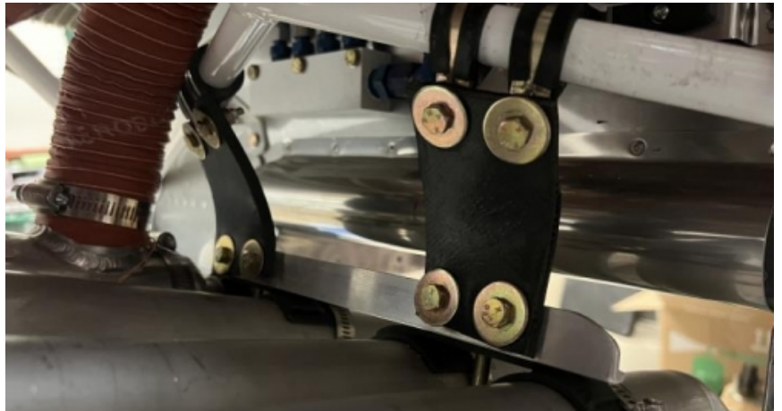
Jim's method for hanging the exhaust on his RV-8
