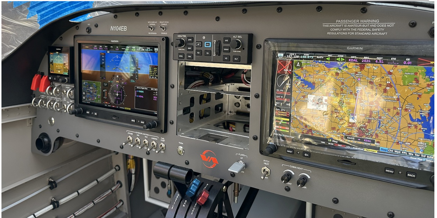
Dual Garmin G3Xs in Greg's RV-10 IFR panel. Missing in the stack is the Garmin Navigator and the radio
