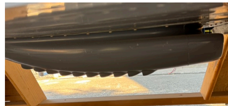
Belly Scoop holding the Condenser section on the RV-10
