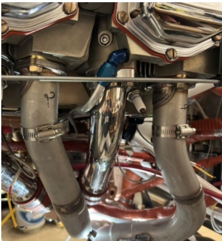
EGT's probes installed in the RV-8's engine
